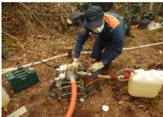
Automatic chemical mixing system (Line proportioner, etc.)
